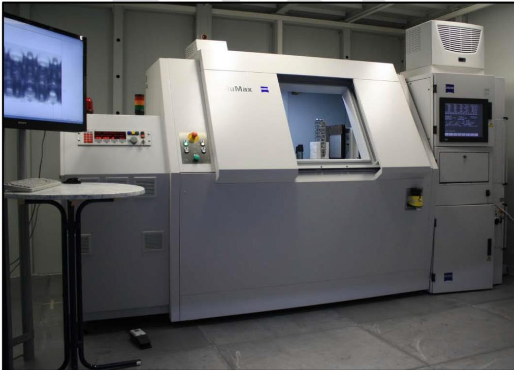
*ZEISS VoluMax 800 CT Machine for High-speed X-Ray Tomography.*
